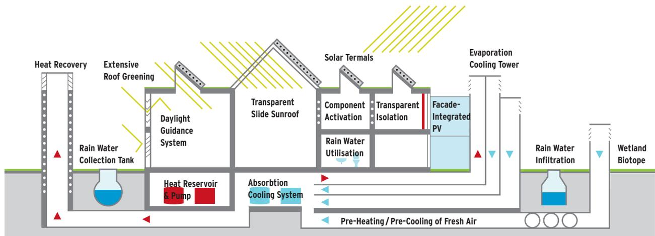
Fig. 4: Design, function and technology- schematic overview of the green building-services systems for the Umwelt-Campus
