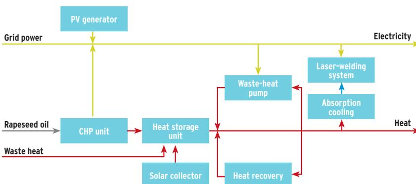
Fig. 5: Schematic overview of the energy-supply network for the Solvis facility
